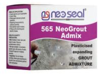
NeoSeal® 565 Plasticised Expanding Grout Admix is a specially formulated grouting aid which is a combination of a plasticizing agent and a gas producing expansion medium. It plasticizes the mix allowing for substantial reduction in water content with maintaining the fluidity, thus improving the strength and water impermeability of the grout. The expansive additives reverse the natural settlement and plastic shrinkage of the grout and aids stability and cohesion.
