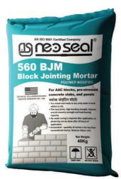
NeoSeal® 560 BJM Block Jointing Mortar is a high-strength adhesive for quick and firm laying of AAC blocks with thin joints. Made of cement, graded sand, and blended with polymers, it provides high strength and water retention properties even when in thickness of 3 mm layer against 12 to 18 mm conventional mortar.
