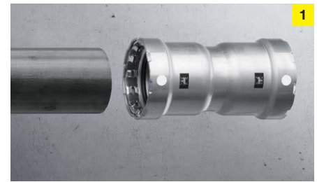
1 The steel pipe is cut to length and cleaned. Then the insertion depth is measured and marked, then the Megapress S connector is put on the pipe up to the mark.
